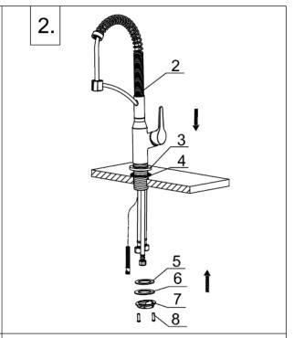
Put main body(2) with washer A(4) and escutcheon(3) through the hole, and then install with washer B(5), gasket (6), nut(7) and screws(8) in sequence from under deck.
