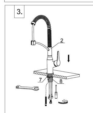
After adjusting to proper position of main body(2), fix it by nut(7) with a wrench, and screws(8) with a Philips screwdriver.
