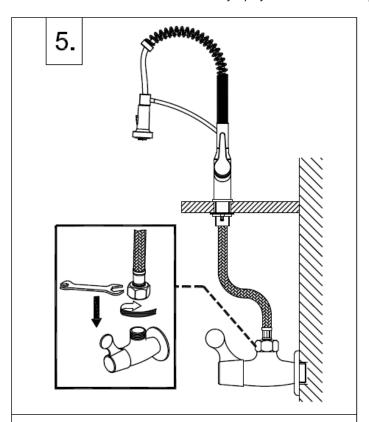
Connect hot and cold water supplying separately with two inlet pipes of main body. Finally, turn on water to test tightness of all joints to finish installation.
