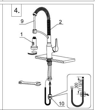
Connect spray head(1) to the pull out hose(9), and connect pull out hose with outlet pipes of main body to make it tight. Fix the back weigth(10) at position of pull out hose as above.
